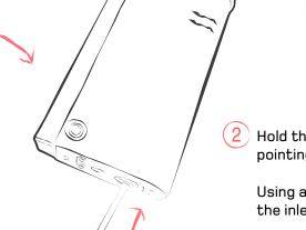
Hold the lighter with the inlet valve pointing downwards.
